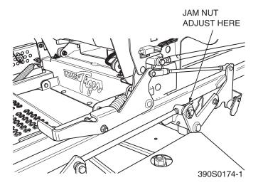
Figure 6-6. Cutter Deck Level Adjustment
